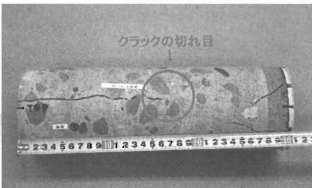
Fig.4 Judged 162mm Crack, Inspected165mm Crack
