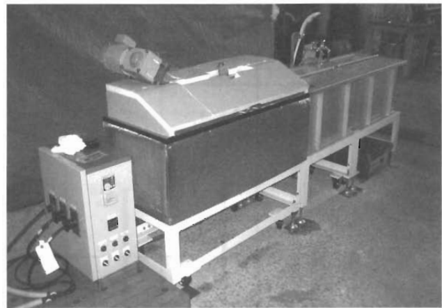
Fig.2.11 Appearance of Chemical Decontamination Test Equipment
